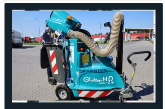
Equipped with an **ergonomic spray gun** that is easy to carry in an integrated handle. with a medium pressure compressor, water tank, pump and filter. The jet pressure can be adjusted on the handle (concentrated or diffused).
